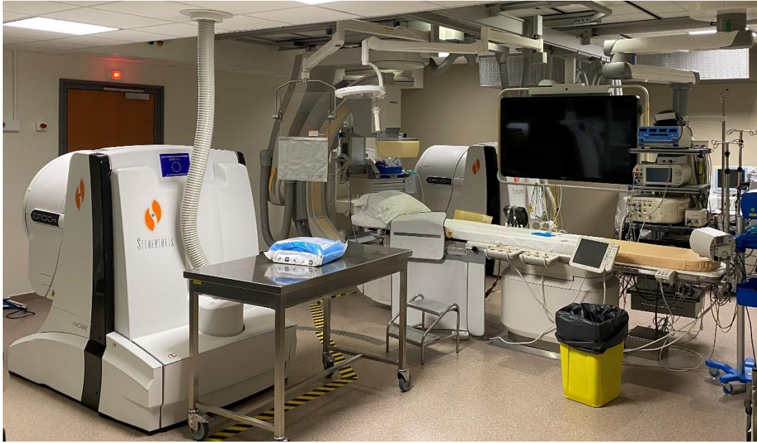
Figure 6. Electrophysiology room in Nancy equipped with the remote magnetic navigation Niobe® system (Stereotaxis Inc., St. Louis, USA). The two permanent magnets are located on both sides of the table.
