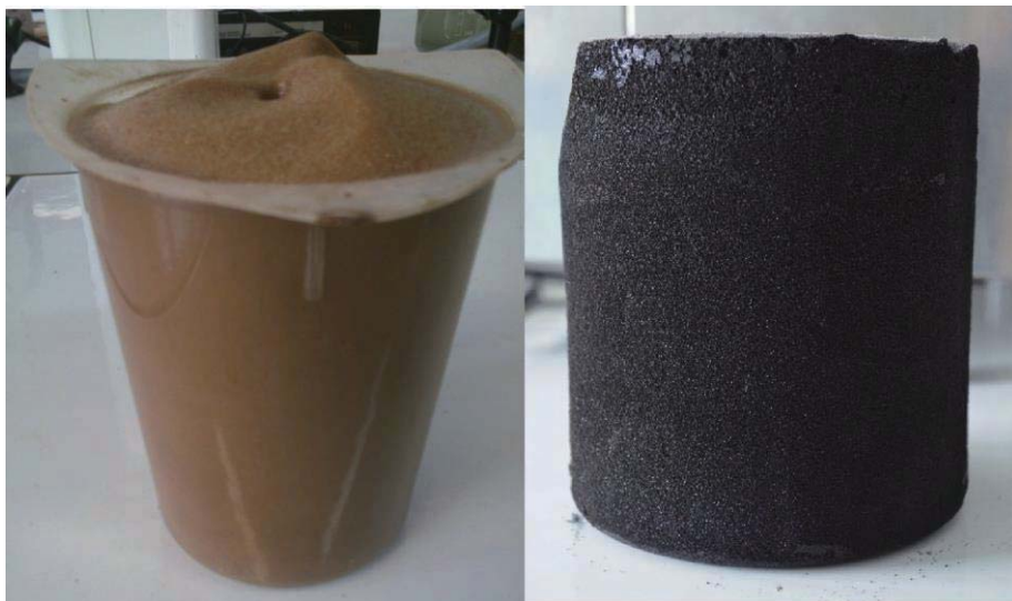
Figure 39 A tannin rigid foam obtained by mechanically blown.
