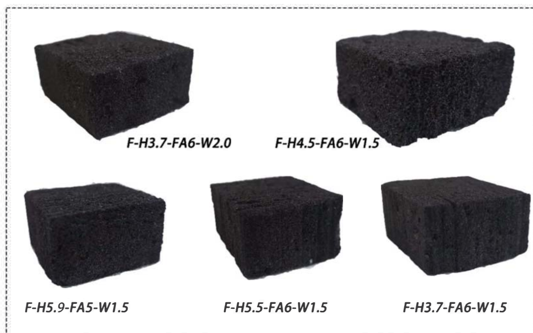
Figure 12. Photographic record of appearance of the experimental tannin–humins foams once cut into cubes.
