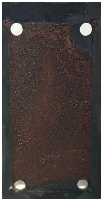
Fig. 61. Scaling on BDD anode after electrooxidation experiments of OMWW.
