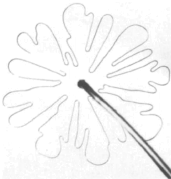
Fig 5.2: Viscous fingering around the injection point observed in Hele-Shaw(L. Paterson, 1983)
