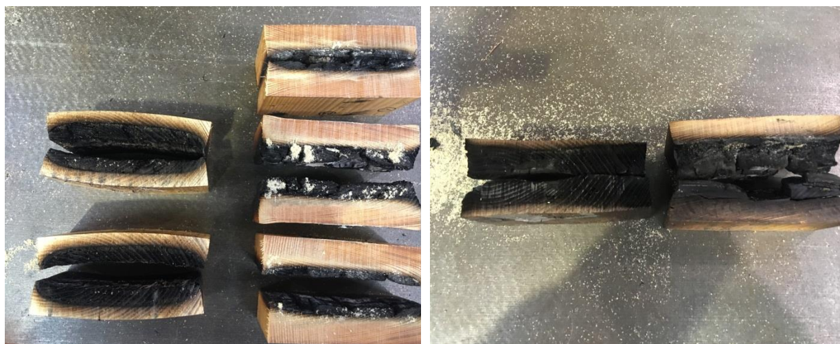
FIGURE 3.21 - The charring depth for virgin and densified spruce after cone calorimeter tests.
