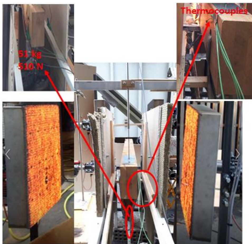
FIGURE 4. 14 - Testing diagram of fire test of connection.
