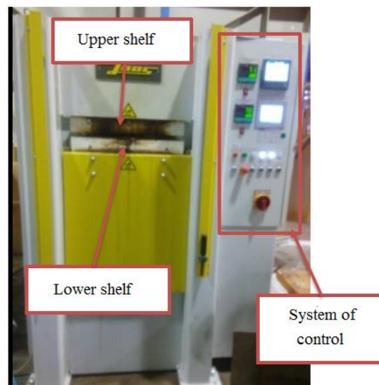
FIGURE 1. 7 - Hydraulic press with heated plates (maximum capacity 1500 kN).
