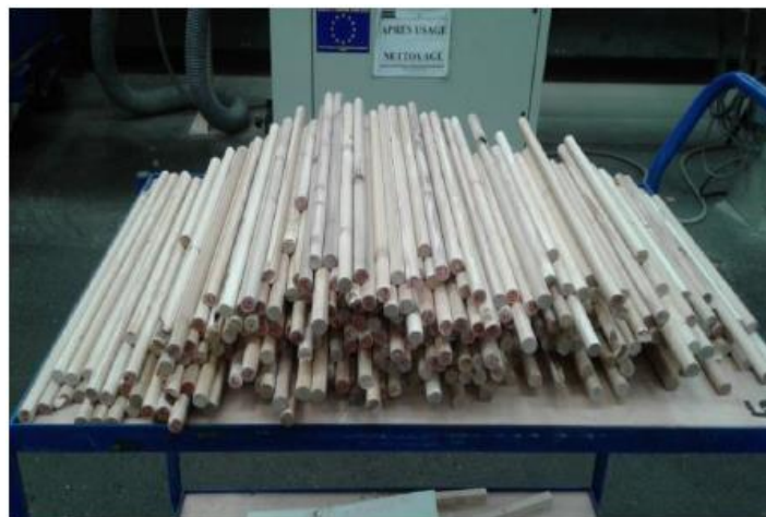
FIGURE 1. 11 - Dowels produced from densified spruce.
