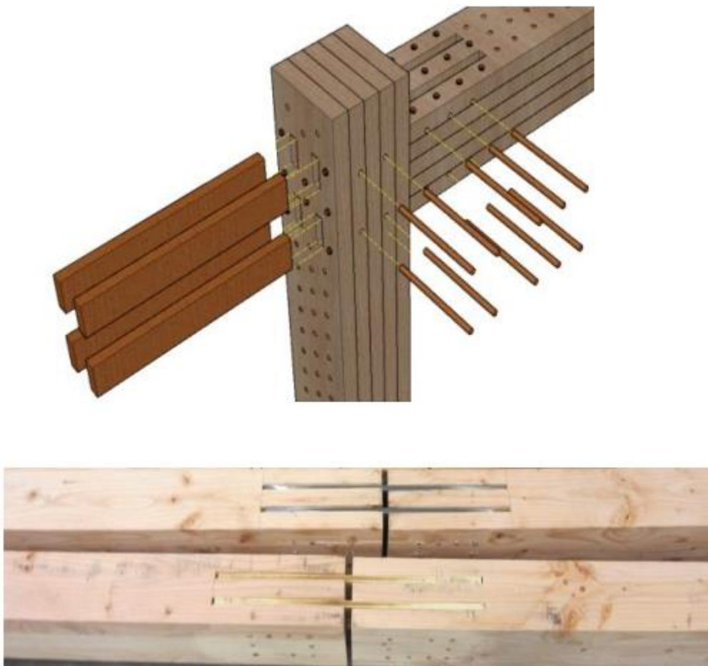
FIGURE A2. 3 - Example of beam-column and beam-beam connections developed at Galway University.
