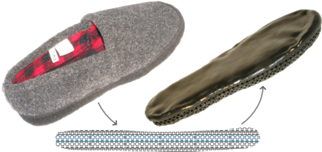
Figure 2.21: An example of real (left) and replicated (right) with a 3D printer objects [24]. The internal structure of the replicated design (bottom) consists of two different materials (black and blue).
