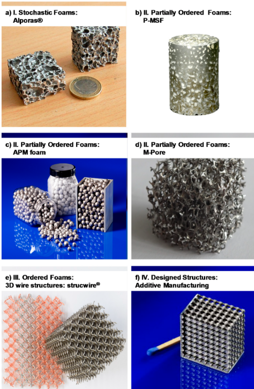
Figure 2.26: Examples of metallic foams corresponding to different manufacturing process and the degree of control over their microscopic structure [114].
