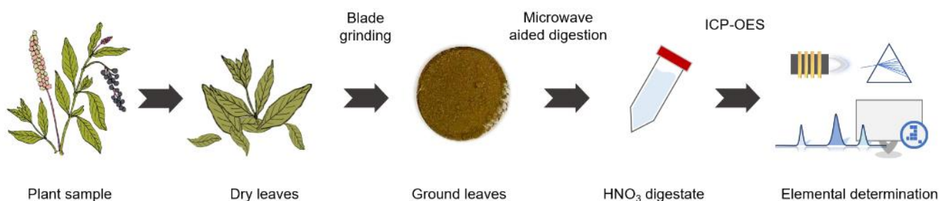
Figure 46: Sample preparation flow in the case of the determination of the elemental composition of dry leaves.
