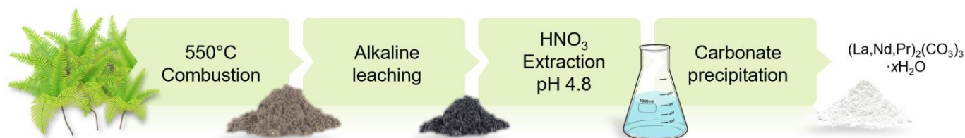
Figure 84: Process developed in this thesis for the recovery of REEs from D. linearis ash
