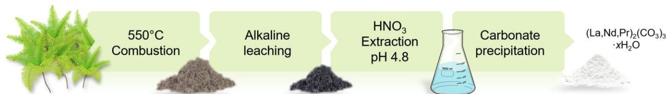
Figure 75: Process developed for the recovery of REEs from D. linearis ash.
