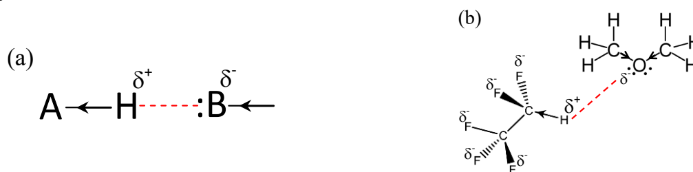
Figure 6.1. (a) Illustration of the definition of a hydrogen bond (red dashed line). The arrows indicate the more electronegative atom, i.e., the direction in which the shared pair of electrons (of the covalent bond) is shifted. (b) case of the pentafluoroethane-dimethyl ether system.
