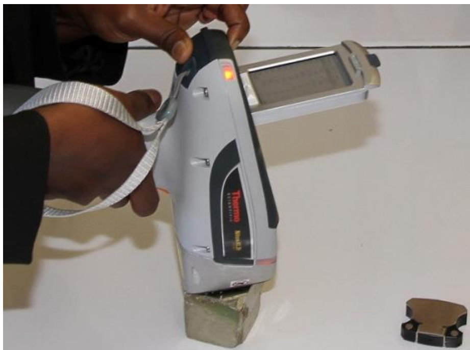
Fig. 8. Thermo Fisher Niton XL3t GOLDD+ XRF analyser.
