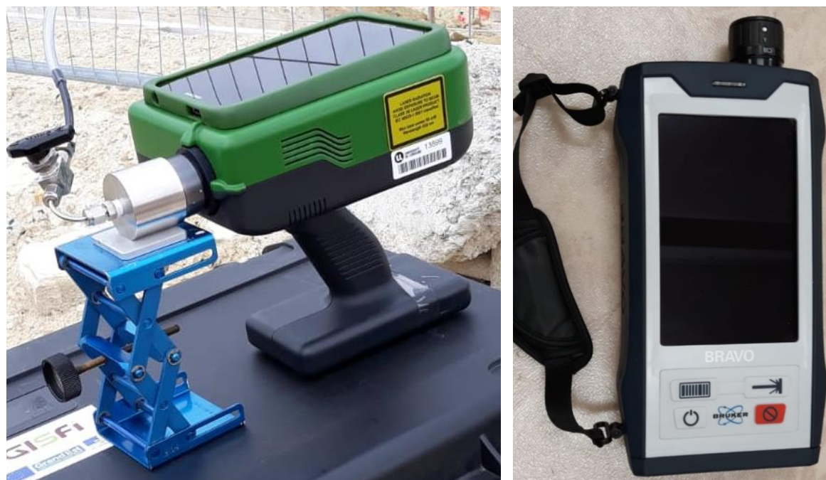
Fig. 17. EnSpectr RaPort Raman spectrometer (left) and Bruker Bravo Raman spectrometer (right).
