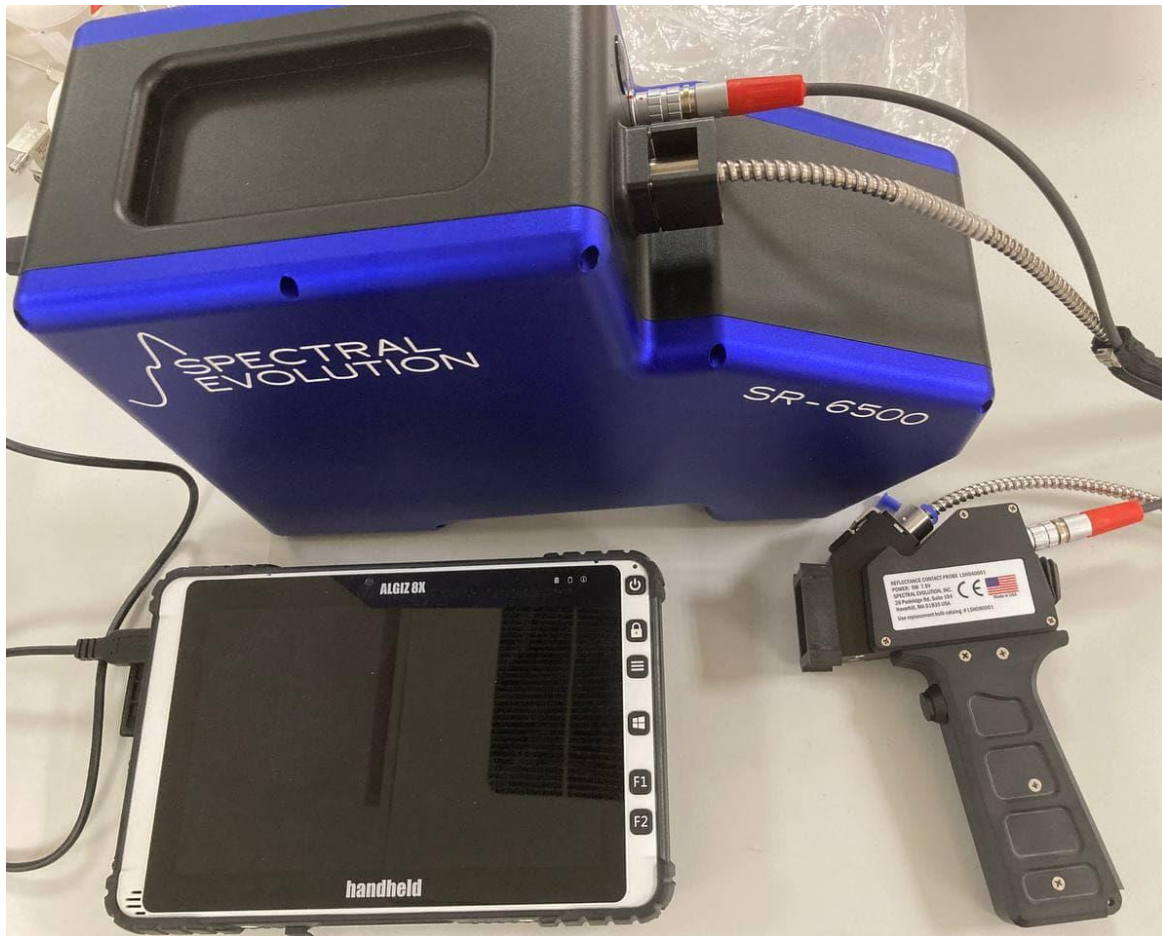
Fig. 14. Spectral Evolution SR-6500 VNIR-SWIR spectrometer.
