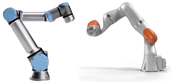
Figure 2.1 UR10e and KUKA LBR IIWA 7 R800 collaborative robots, using Harmonic Drive gearboxes
