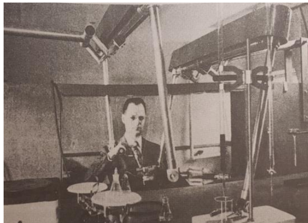
Figure 1.2 First mechanical telemanipulation system
