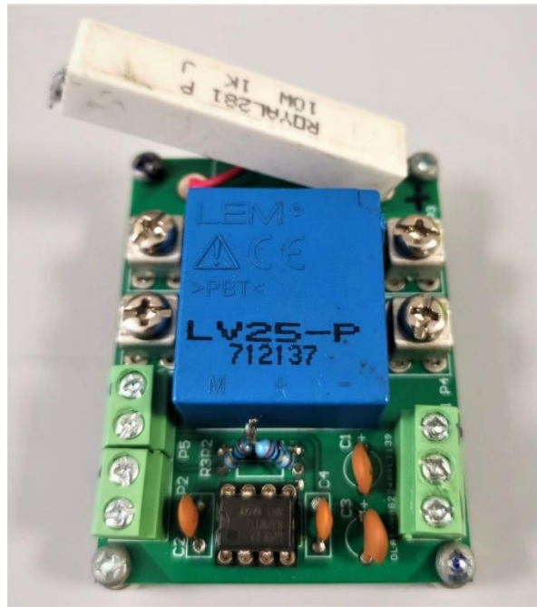
Figure 4-4: Implemented voltage sensor.
