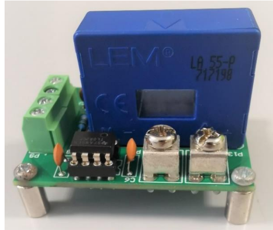
Figure 4-6: Realized current sensor.
