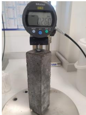
Figure 2.7 Standard mortar mounted in an extensometer
