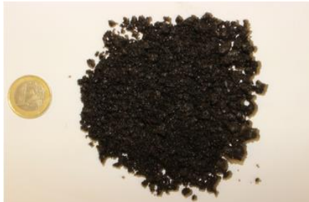
Figure 2.3 Picture of the fumed fayalite slag sample as received
