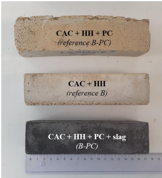
Figure 5.2 Pictures of the B-PC and B (high-sulfate) mortars after 45 days of curing under water
