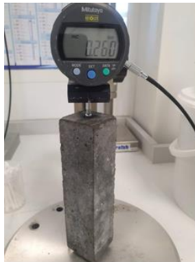
Figure 2.7 Standard mortar mounted in an extensometer
