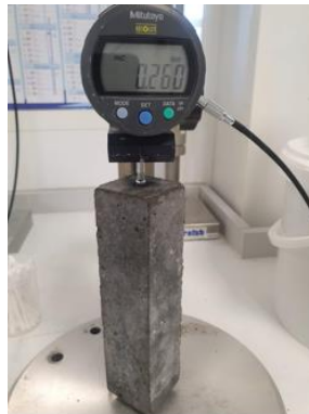
Figure 2.7 Standard mortar mounted in an extensometer
