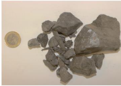
Figure 2.2 Picture of the slowly-cooled Fe-rich slag sample as received
