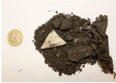
Figure 2.4 Picture of the MSWI bottom ash sample as received
