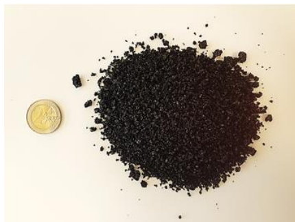
Figure 2.1 Picture of the granulated Fe-rich slag as received
