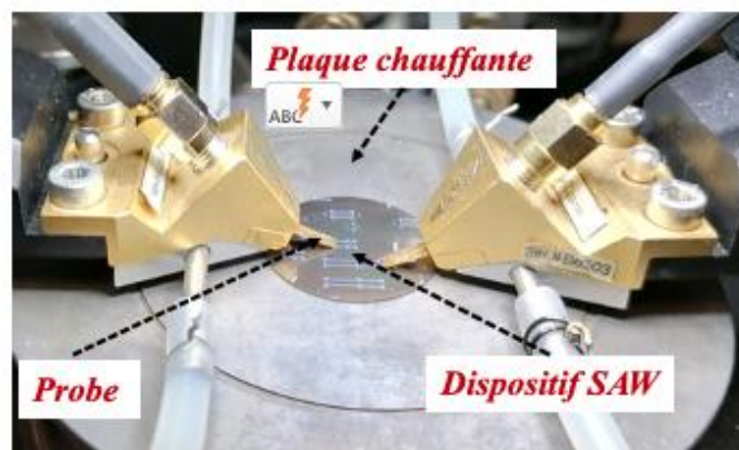
Figure 3. 18 : Station sous pointe S-1160, Signatone
