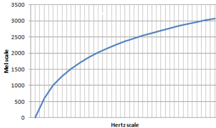
Figure 2.5 – Mel scale plot stating equally spaced intervals of frequencies perceived by human ear, where horizontal axis are linear Hz frequencies, and vertical axis are Mel frequencies.
