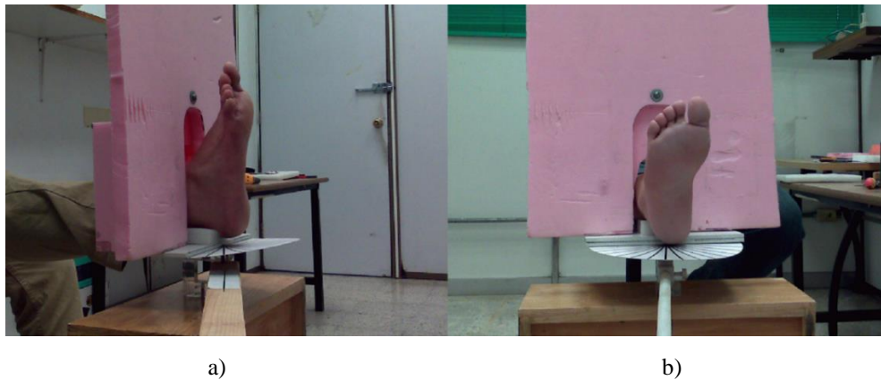
Figure 43: Foot posture during the image acquisition. a) Lateral view of the foot on the resting base. b) Frontal view. It is noteworthy that the pink background foam is large enough to isolate the foot from the remaining body of the volunteer so that the IR radiation does not interfere with the captured frame.
