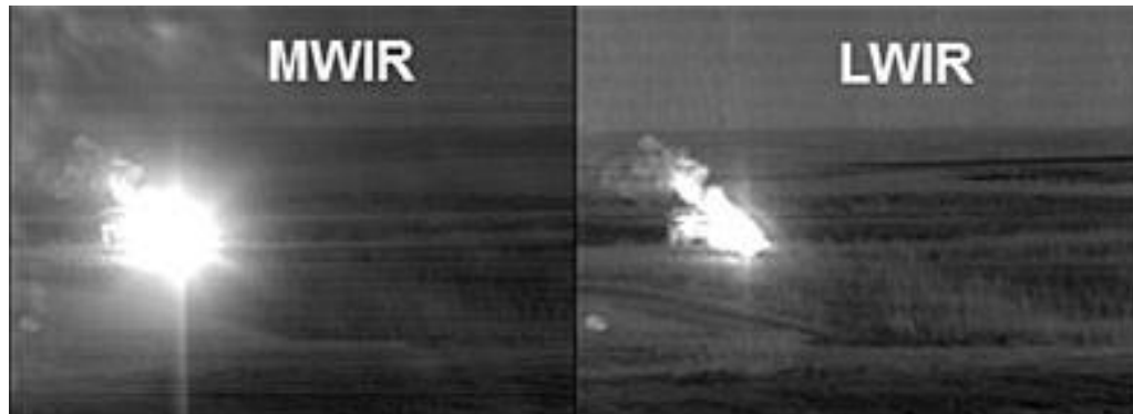
Figure 15: In certain scenarios, such as when there are hot targets, LWIR can outperform MWIR. Burning barrels, as illustrated in this figure, is a clear demonstration of the LWIR advantage. With large energy in the MWIR, hot targets shift left on Planck's curve, yet the LWIR image remains functional with burning barrels in the field of view [116].
