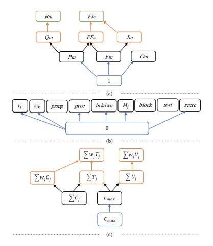
Fig. 1.2 Complexity hierarchies of deterministic scheduling problems: (a) Machine environments (b) Processing restrictions and constraints (c) Objective functions [48]
