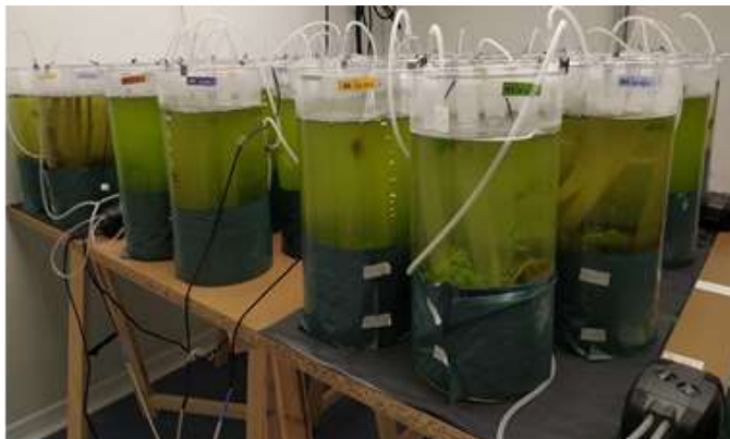
Fig. 2.5. Photo of microcosms in Experiment 2. Microcosms on the left and right are placed above heating mats and represent the heated treatments. Phytoplankton development is visible. Plastic strips were hung vertically by attaching to a pipette placed horizontally over the rim of the glass cylinders. The lower ends of the cylinders were covered in black plastic to mimic light exposure in real lakes.
