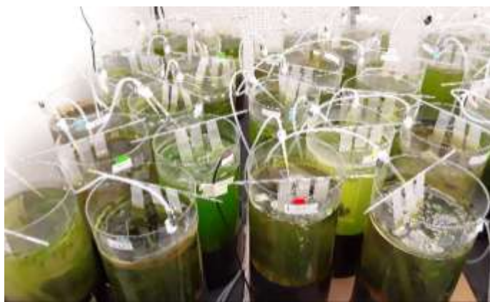
Fig. 2.4. Photo of microcosms in Experiment 1. Plastic strips were hung vertically by attaching to a pipette placed horizontally over the rim of the glass cylinders. The lower ends of the cylinders were covered in black plastic to mimic light exposure in real lakes.
