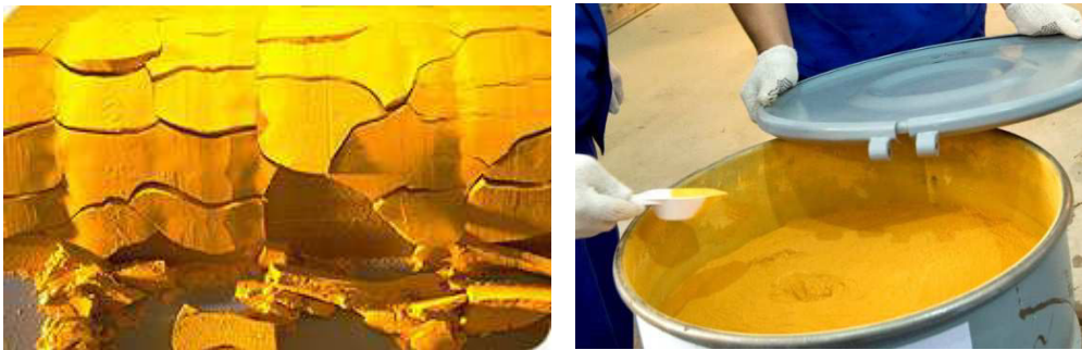
Figure 1.5 – Filtration du Yellow-cake (gauche) et baril de Yellow-cake (droite)
