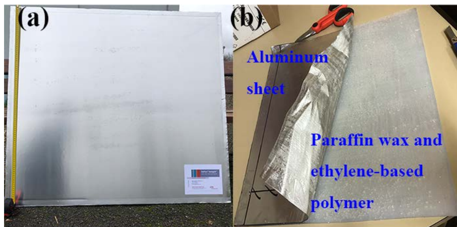
Fig. 3.1. Finished shape-stabilized PCM: (a) PCM panel; (b) aluminum sheet and the mixture of paraffin wax and ethylene-based polymer
