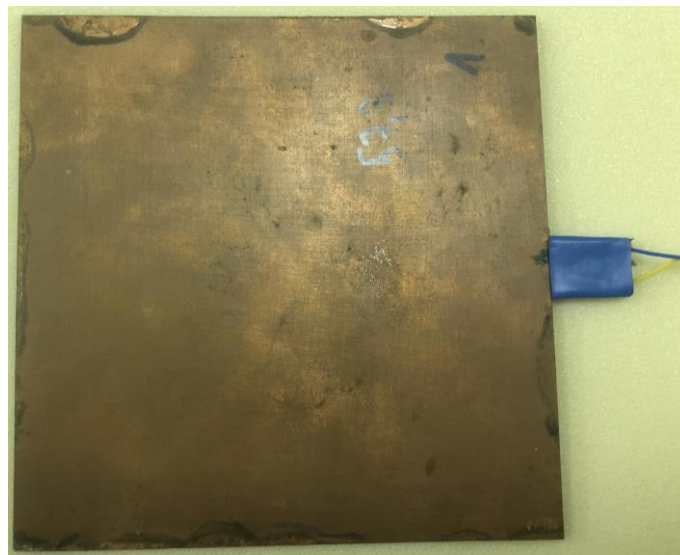
Fig. 3.6 Heat flux sensor
