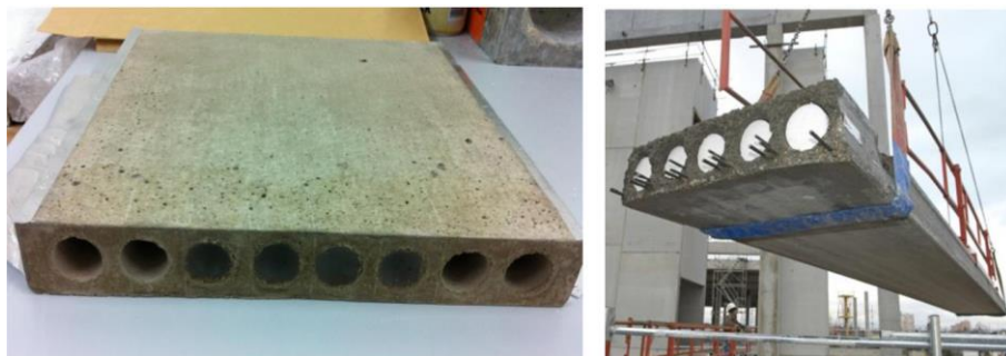
Fig. 2.11. Floor panel incorporated with PCM [142]
