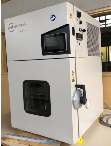
Fig. 3.4 Climatic chamber (LabEvent L C/64/40/3)
