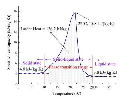
Fig. 3.2. Specific heat capacity of the PCM [222]
