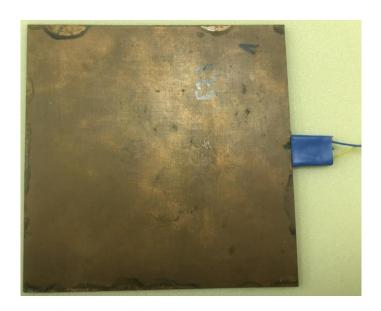
Fig. 3.6 Heat flux sensor
