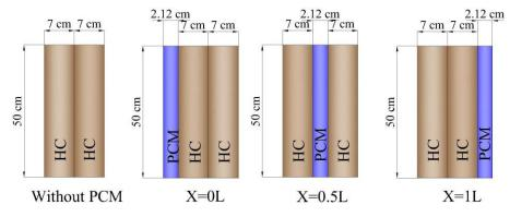
Fig. 3.9 Four envelope configurations of integrating HC and PCM
