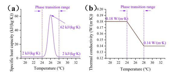
Fig. 4.2. Thermal properties of PCM: (a) specific heat capacity; (b) thermal conductivity
