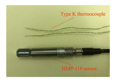
Fig. 3.5 Type K thermocouple and HMP-110 sensor
