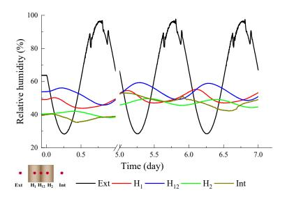
In this research, the points close to the indoor side ( $H_{12}$  and especially  $H_2$ ) are the main interest to us, because their temperature and relative humidity behavior influences indoor hygrothermal comfort. Therefore, the temperature and relative humidity behavior of  $H_{12}$  and  $H_2$  will be the focus of the following sections.
