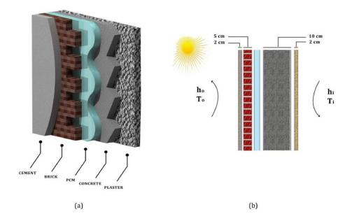
Fig. 2.10. Schematic diagram of a PCM wallboard [140]
