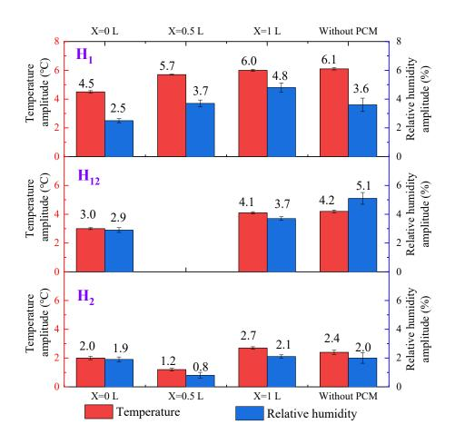
Fig. 3.33. Temperature and relative humidity amplitudes of HC in different configurations
