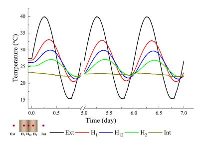
Fig. 3.25. Temperature behavior of the configuration without PCM
