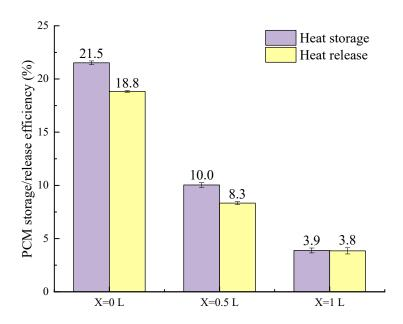
Fig. 3.38. PCM's storage/release efficiency
