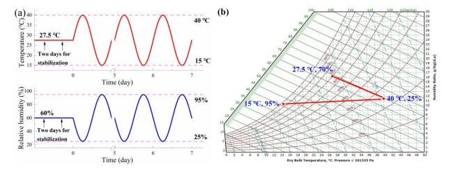
Fig. 3.13 Dynamic boundary condition: (a) temperature and relative humidity condition provided by the climatic chamber; (b) temperature and relative humidity in the psychrometric chart
