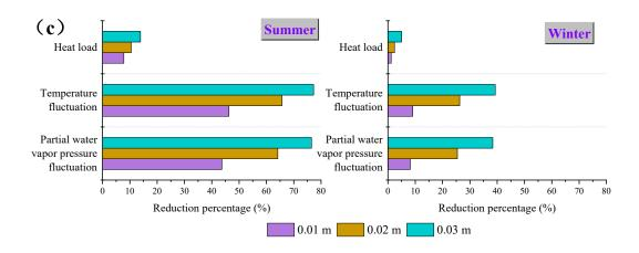
Fig. 5.2. Impact of PCM thickness: (a) cumulative heat load and moisture load; (b) variation of temperature and partial water vapor pressure; (c) reduction of heat load, temperature fluctuation, and partial water vapor pressure fluctuation compared to configuration baseline
