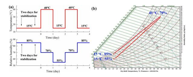
Fig. 3.12 Static boundary condition: (a) temperature and relative humidity condition provided by the climatic chamber; (b) temperature and relative humidity in the psychrometric chart
