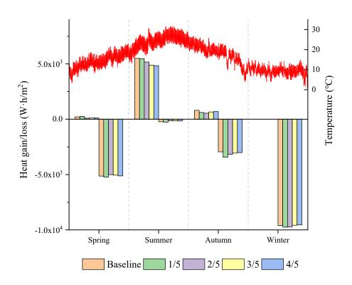
Fig. 4.10. Annual heat load for different configurations
