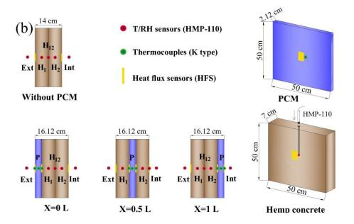
Fig. 3.10 Monitoring points for temperature, relative humidity, and heat flux of (a) configuration X = 0 L in full view and (b) all the configurations
