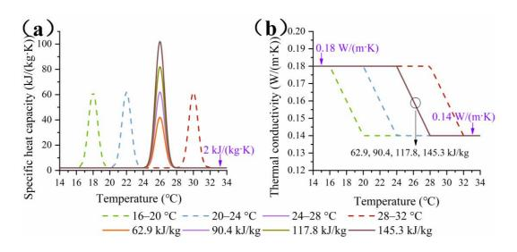
Fig. 5.1. Thermal properties of PCMs with different phase transition ranges and latent heats: (a) specific heat capacity; (b) thermal conductivity
