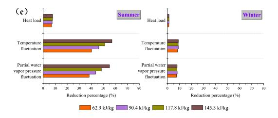
Fig. 5.3. Impact of PCM latent heat: (a) cumulative heat load and moisture load; (b) variation of temperature and partial water vapor pressure; (c) reduction of heat load, temperature fluctuation, and partial water vapor pressure fluctuation compared to configuration baseline
