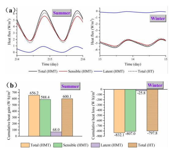
Fig. 4.6. Comparison between HMT and HT models: (a) heat fluxes; (b) heat loads
