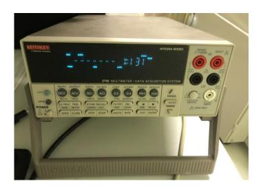
Fig. 3.7 Keithley 2700 date acquisition equipment
