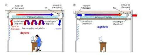
Fig. 2.13 Ventilated cooling ceiling with PCM [150]
