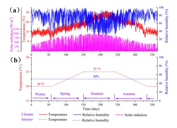
Fig. 4.4. Annual climate and interior conditions: (a) exterior climate in Rome; (b) interior temperature and relative humidity
