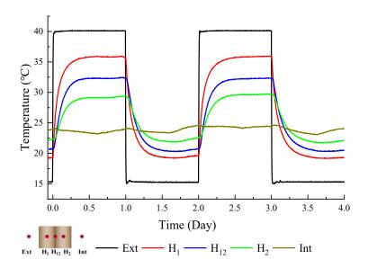
Fig. 3.14 Temperature behavior of configuration without PCM
