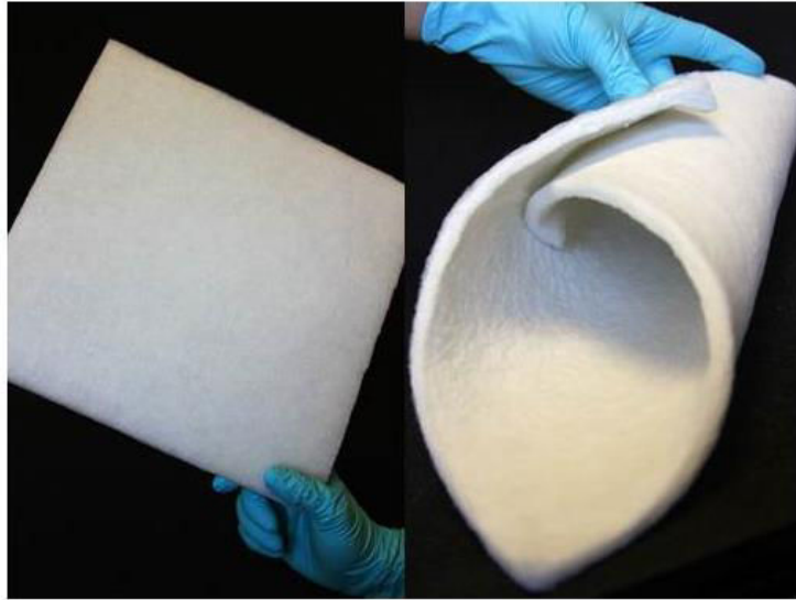
Figure 4.9. Inorganic aerogel board (left) and blanket (right).
