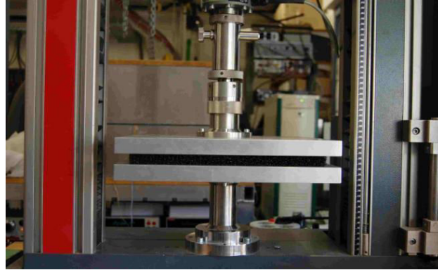
Figure 3.6. Experimental setup for compression testing with two parallel plates. (ZAE)
