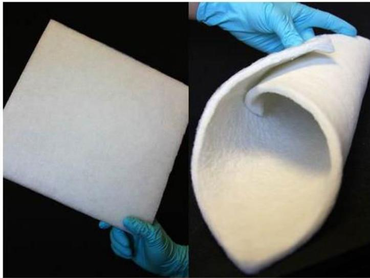
**Figure 4.9.** Inorganic aerogel board (left) and blanket (right).
