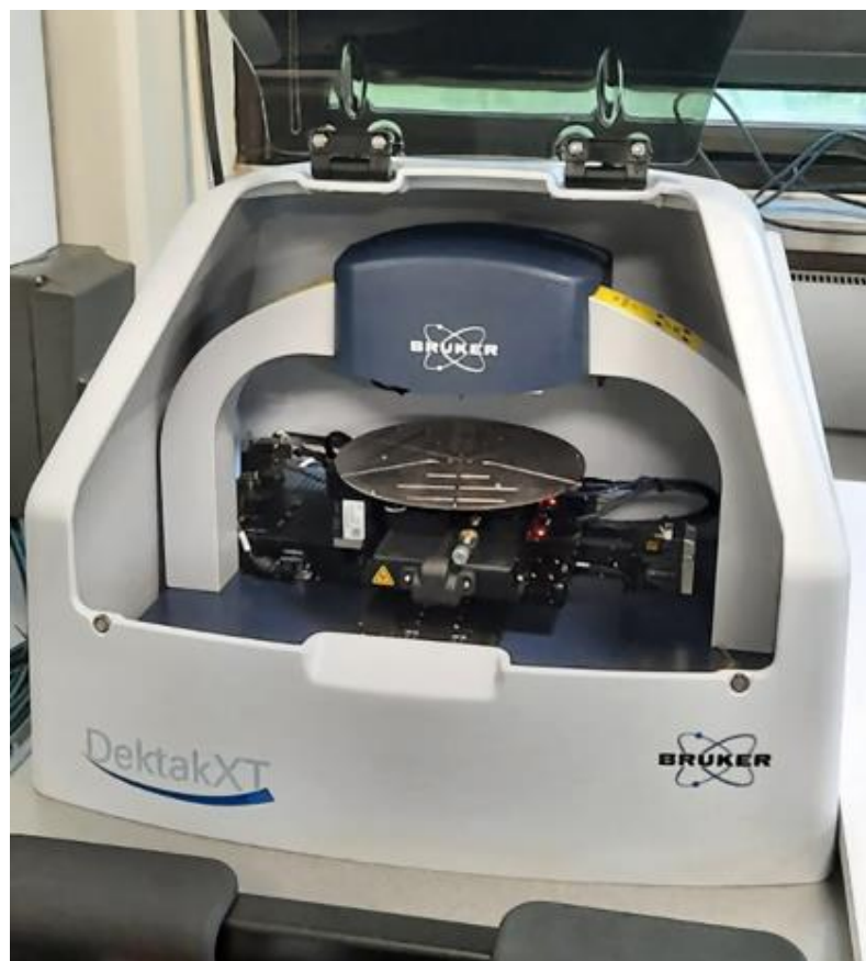
Figure 2.12: Dektak XT mechanical profilometer from Bruker available at LMOPS laboratory.
