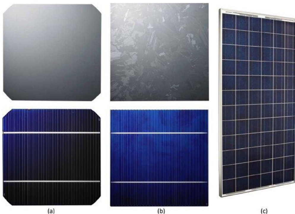
Figure 1.11: Three types of silicon wafers for solar cells: (a) 156-mm monocrystalline solar wafer and cell; (b) 156-mm multi-crystalline solar wafer and cell; and (c) 280-W solar cell module (from multi-crystalline wafers) [63].
