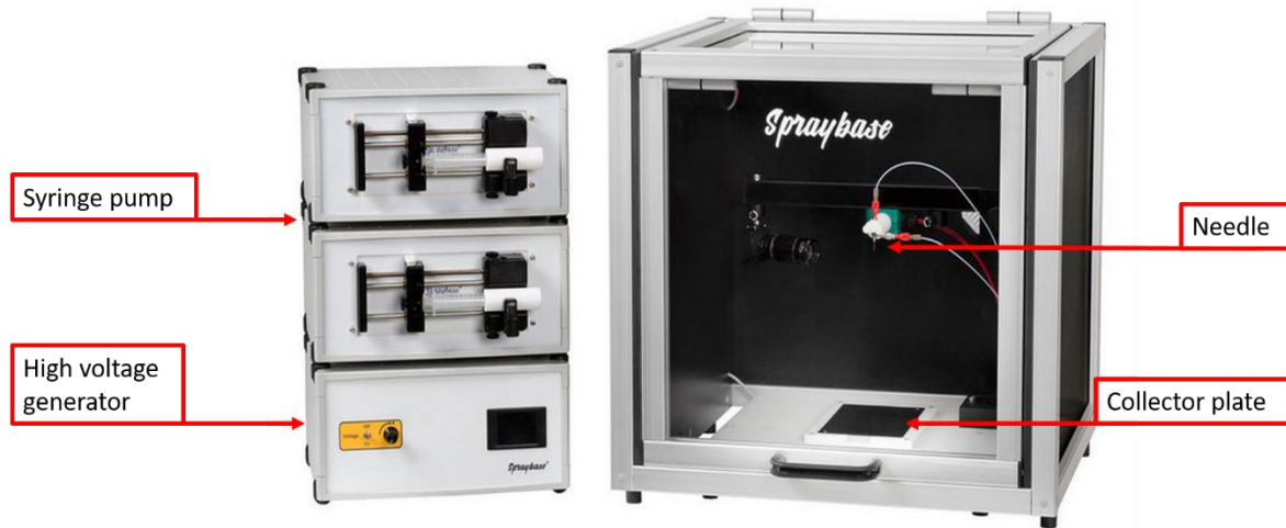
Figure III. 5. Electrospinning machine used during my thesis at LMOPS.
