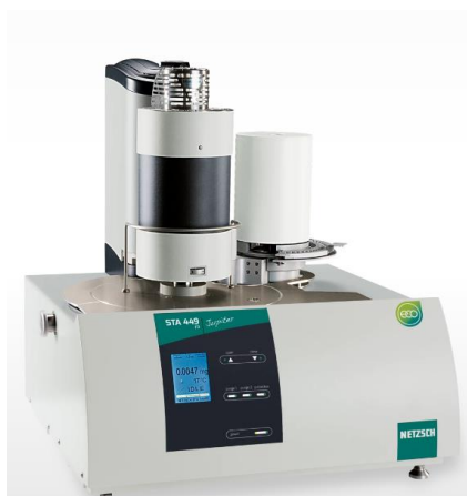
Figure IV. 6. Apparatus used for TGA-DSC analysis of nanofibers at LERMAB.
