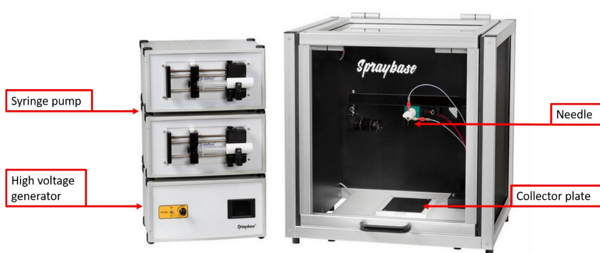
Figure III. 5. Electrospinning machine used during my thesis at LMOPS.
