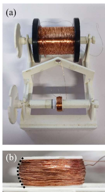
FIG. 4.12. (a) The winding tools. (b) The arc-like coil sample.
