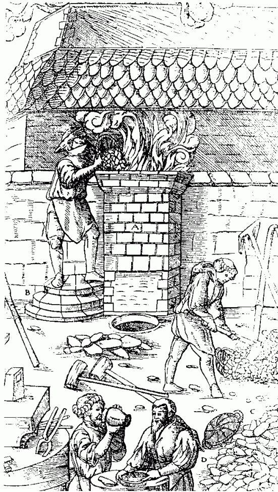
Figure 19. Bloomery for making wrought iron [76]
