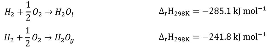
If all this energy could contribute to the production of electricity, a theoretical voltage  $E^{TH}$  could be defined as:
