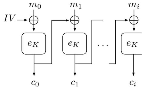
Figure 2.3: Encryption in the CBC mode of operation.
