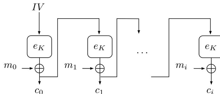
Figure 2.4: Encryption in the CFB mode of operation.
