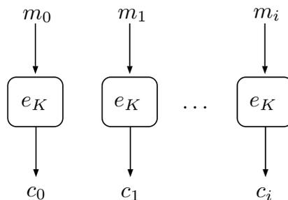
Figure 2.2: Encryption in the ECB mode of operation.
