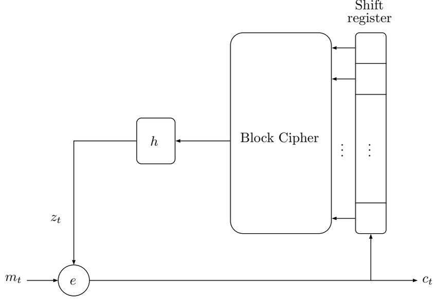
Figure 2.10: SSSC in CFB mode. A shift register is used to gather the previous ciphertexts. The output of the block cipher is filtered with a function  $h$  to produce a 1-bit keystream  $z_t$  that is XORed to the plaintext  $m_t$ .
