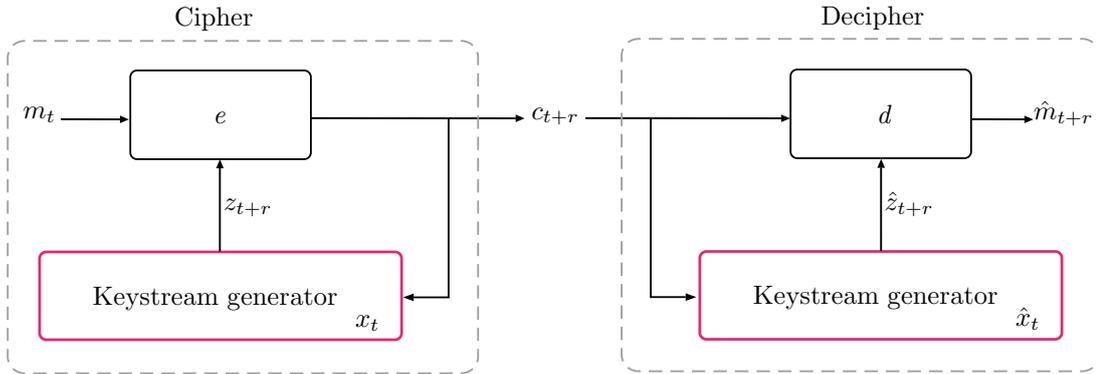
Figure 2.13: Flat LPV-based Self-Synchronizing Stream Ciphers block diagram.
