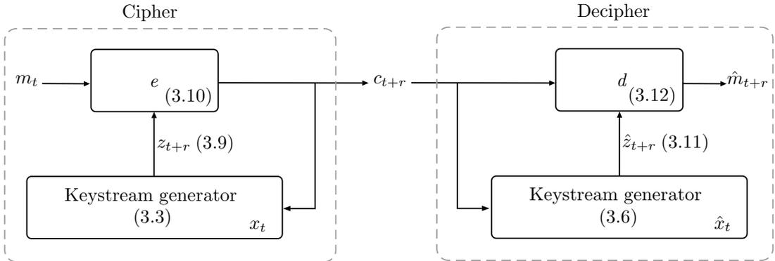
Figure 3.9: Flat LPV-based Self-Synchronizing Stream Ciphers block diagram.
