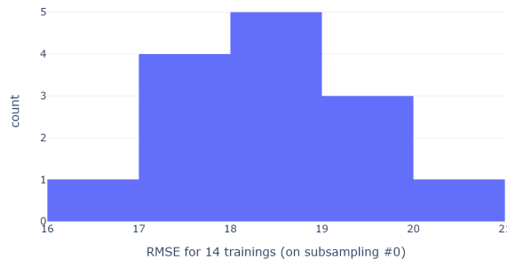
Figure 2.2: Histogram of prognostics performances on a sub-samplings of a full dataset. The dataset is the C-MAPSS FD001, the model used is MiniROCKET, both described in 2.3. Sub-samplings size is 10%.
