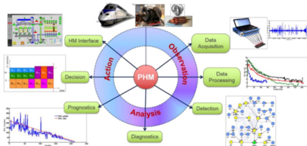
Figure 1.6: Illustration of the PHM processes. Source of the image Atamuradov et al. 2017.
