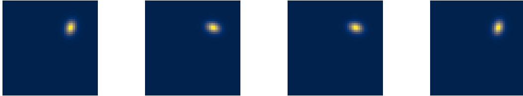
Figure 4.5.: Galaxy data augmentation. The original image, of size 256x256, is cropped at its center in an image of size 64x64. Then, the image is cropped 4 times differently by taking the 45x45 subimage at each corner, and each cropped image is rotated such that each galaxy is in the same quadrant. Each cropped image is used during training (see also Dieleman et al. (2015)).
