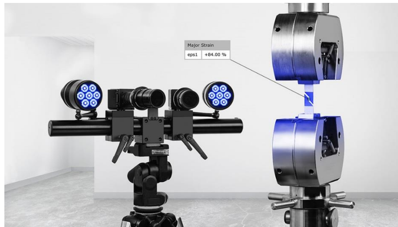
Figure 81: ARAMIS system in front of a tensile tester, as exposed on the constructor website [184].
