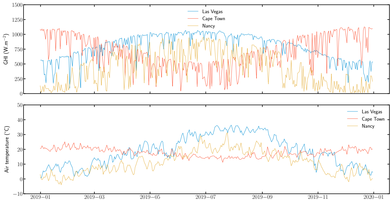
FIG. D.4 : Weather data (global horizontal irradiance, air temperature and wind speed) for 2019 for Las Vegas, Cape Town and Nancy. For the radiation data the daily maximum is displayed and for the air temperature the daily average is plotted.
