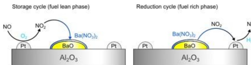
Figure 6.4: Schematic representation of the NO x storage reduction process (NSR). Figure adapted from ref 323 .
