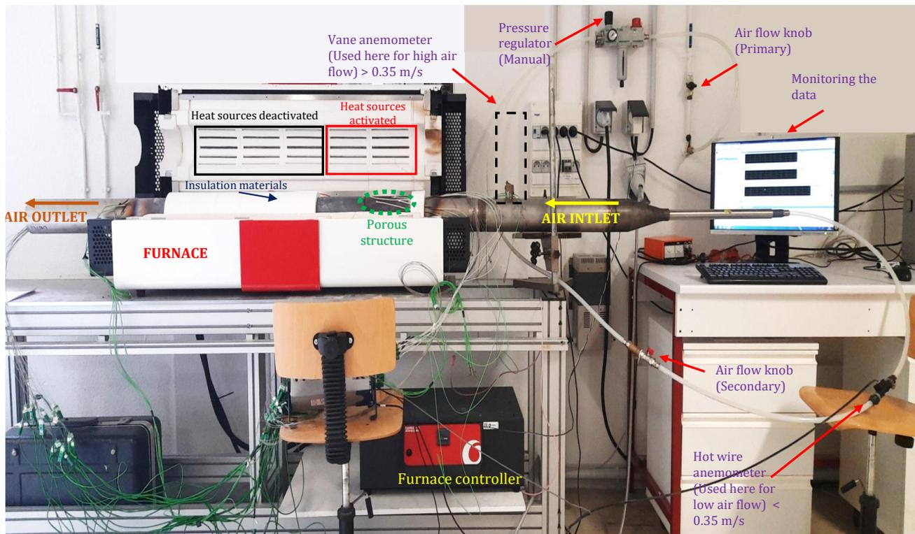
Figure 2.24: Real view - Porous heat exchanger experiment
