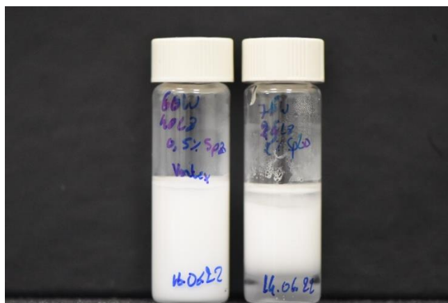
Figure 9: Image of a 60W/40L8 Span 80 0.5% emulsion and another at 70W/30L8 2% Span 80.
