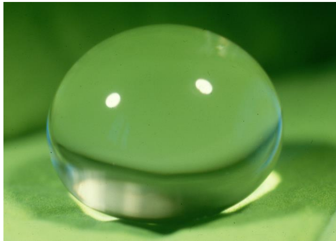
Figure 1: A drop of rain on a lotus leaf (hydrophobic surface)
