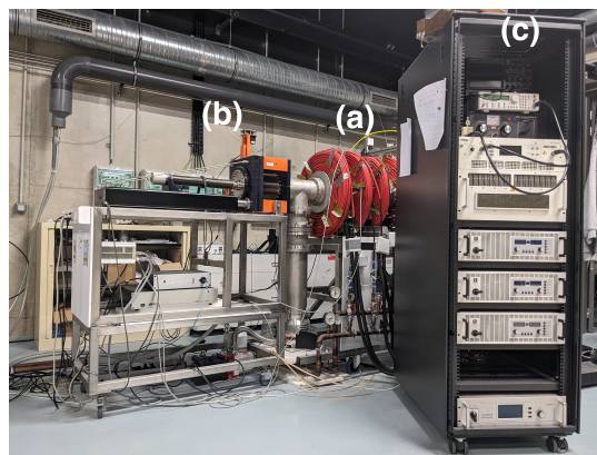
Figure 2.1: Sketch (top) and picture (bottom) of the ALINE plasma device (a), 3D probe manipulator (b) and rack holding the RF power generator, amplifier and coils power supplies (c)
