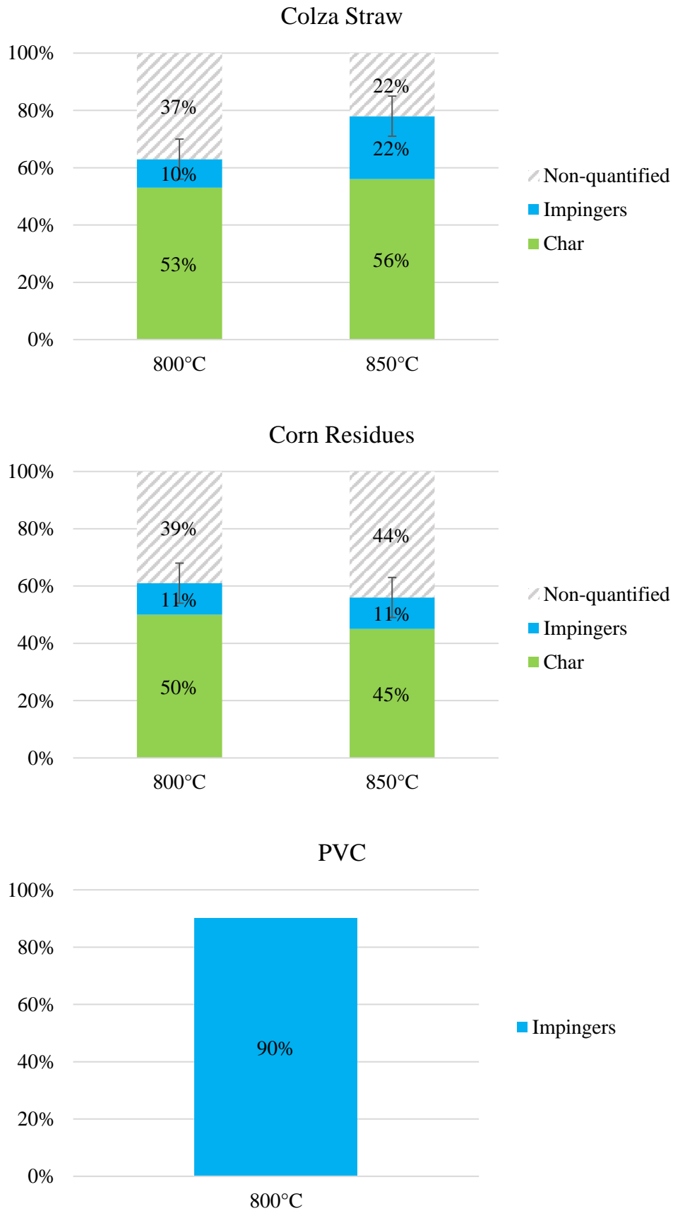
Figure 22: Experimental chlorine distribution in the char and the impingers for the pyrolysis of colza straw, corn residues, and PVC at 800°C and 850°C.
