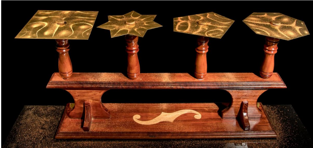
Figure 2 : Figures de Chladni [38]
