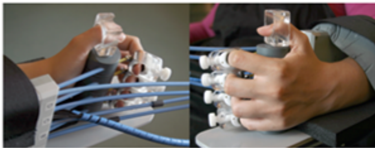
Figure 2.4: Hand exoskeleton developed by Ramos-Murguialday et al. [3]
