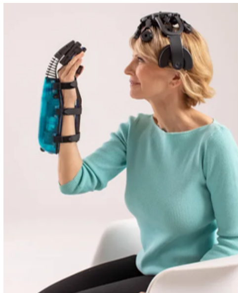
Figure 2.5: Neuroolution's IpsiHand for post-stroke recovery. The system consists of a BCI with proprioceptive feedback from an exoskeleton that can be employed at the patient's home. Extracted from: https://www.neuroolutions.com/
