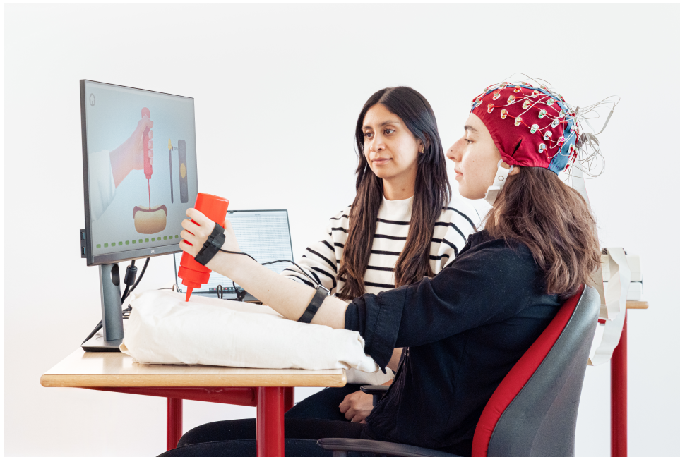
Figure 6.4: The participant is comfortably seated on a chair, holding a bottle with the non-dominant hand. The vibrotactile device is placed on the non-dominant limb and a cushion is placed underneath to avoid dispersing the vibration on the table. The screen displays the visual animation and the brain activity is recorded with a 64-electrode EEG cap and a Biosemi Active Two system.
