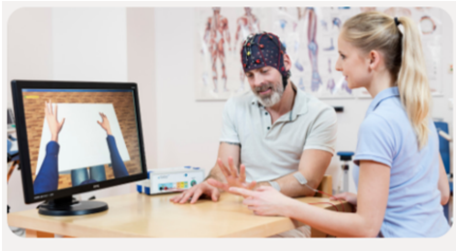
Figure 2.7: g.tec’s recoveriX BCI system for post-stroke motor rehabilitation with visual and FES feedback.
