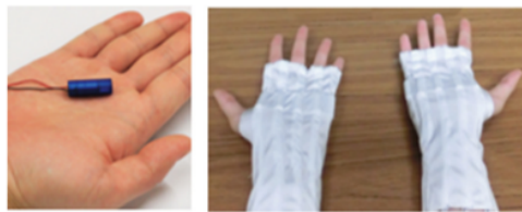
(c) Vibrotactile motors placed on the hand, extracted from [42]
