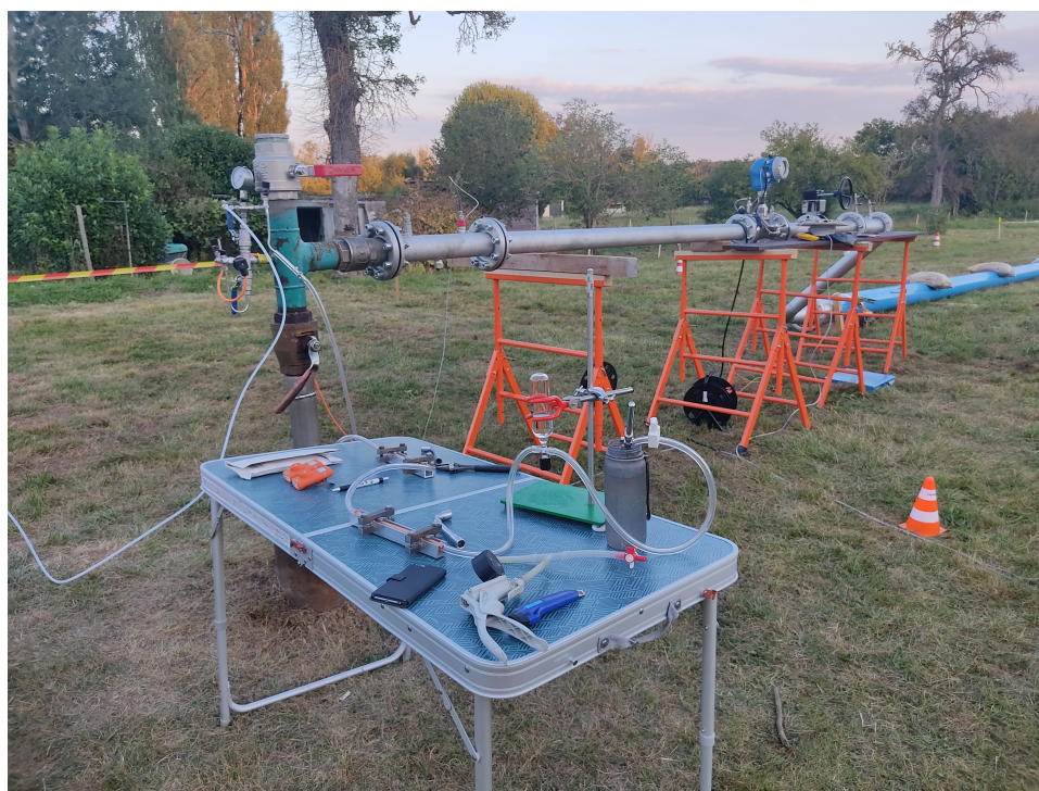
Figure 1.16: Sampling station at the SP4 well. Cu tubes and Giggenbach bottles were connected to the same sampling train to avoid air contamination.
