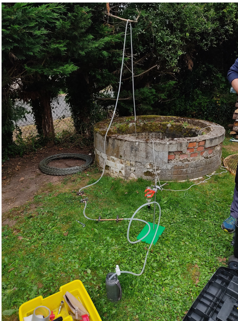
Figure 1.17: Sampling of gelin spring. Cu tubes and Giggenbach bottles were connected to the same sampling train to avoid air contamination.
