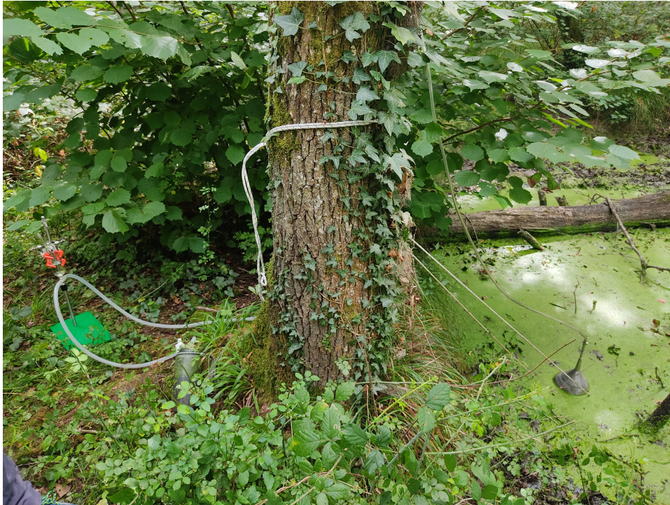
Figure 2.3: Sampling at Fontaine des Vertus, Central France. The funnel is connected to the sampling containers by hoses.
