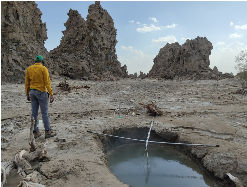
Figure 2.4: Sampling at GVS4, Djibouti. The funnel is connected to the sampling containers by hoses.
