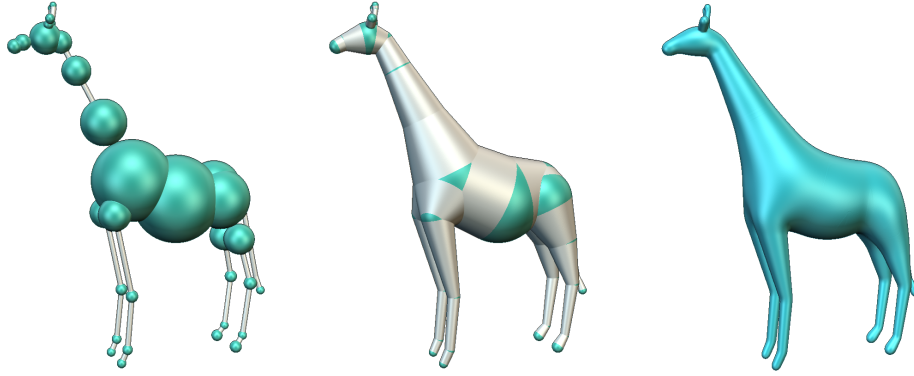
Figure 1.7: Left : a skeleton with prescribed radius on its vertices, Middle : infinite union of spheres defined by linear interpolation of prescribed radius along skeleton edges (union of sphere-cones), Right : resulting scale-invariant integral surface which can be seen as a smoothing of the sphere-cone union.
