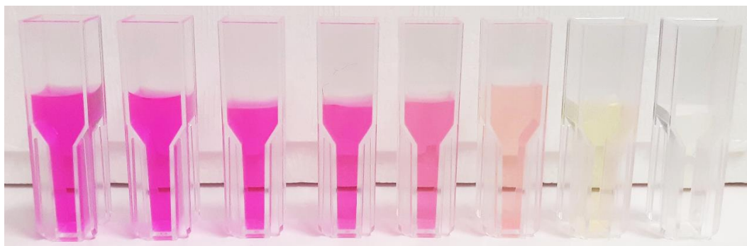
Supplementary Material S4.5: Evolution of RhB solution after exposure duration of 0, 30, 60, 90, 120, 150, 180 and 210 min respectively
