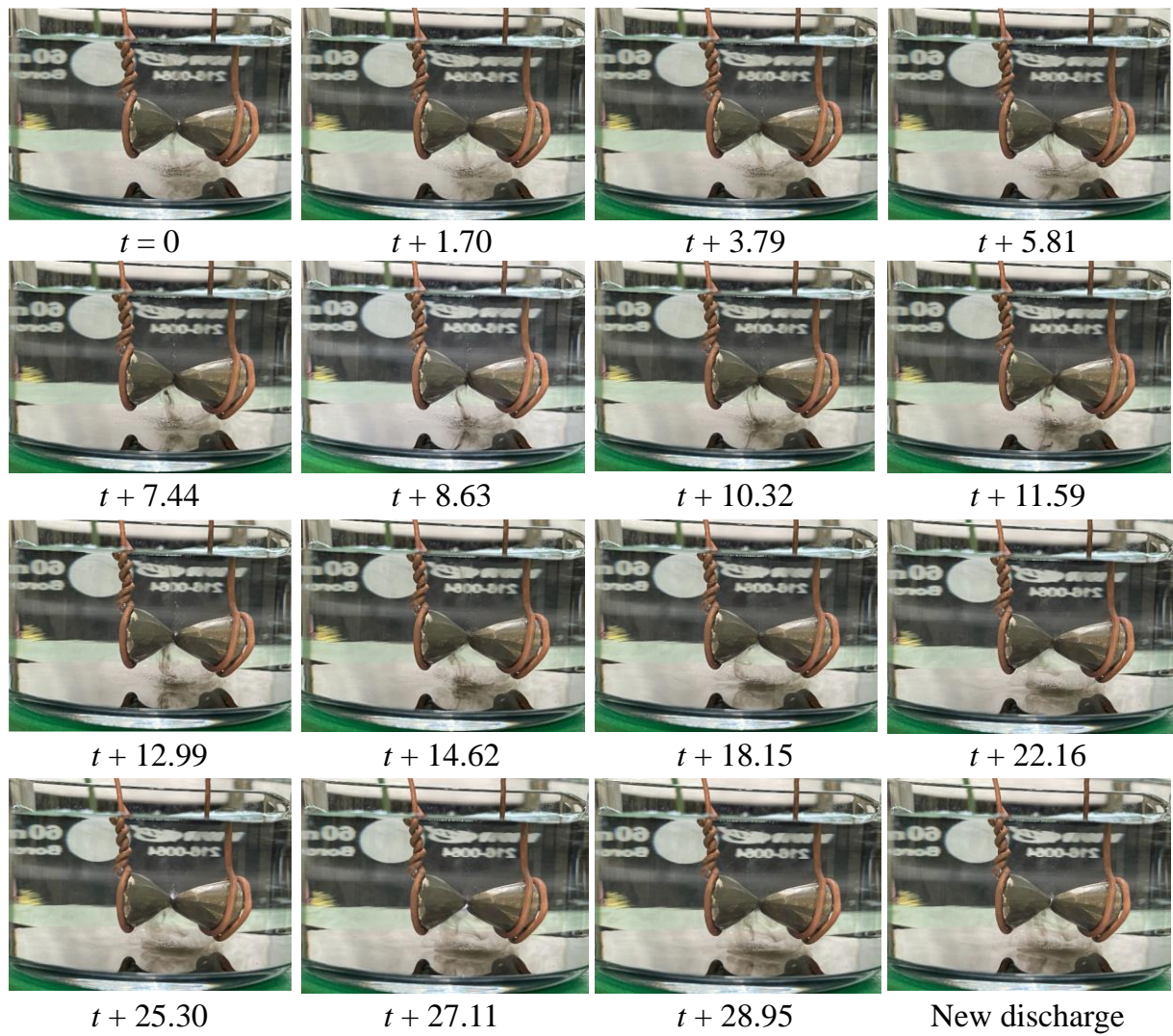
Supplementary Material S2.8: Set of pictures showing the movement of the generated particles in the liquid between two discharges. The time scale is in second. Particles remain at the bottom of the beaker, settling by gravity.
